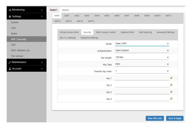
Figure 34. Static WEP in the VAP Security Tab
