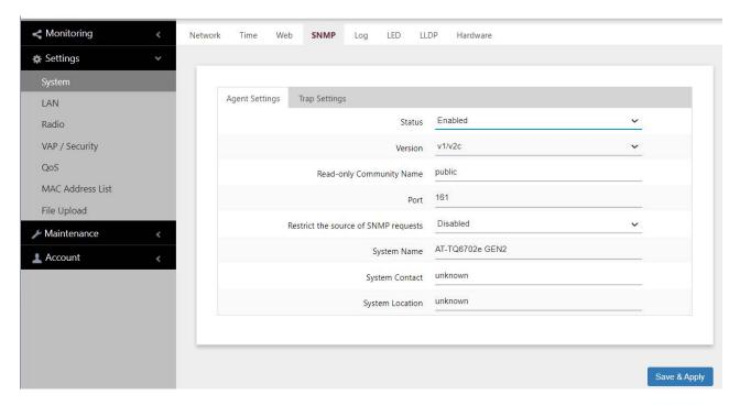
Figure 18. SNMP Window - SNMP Enabled
