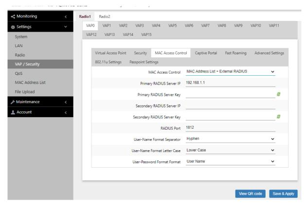
Figure 45. MAC Access Control - MAC Address List + External RADIUS Window
