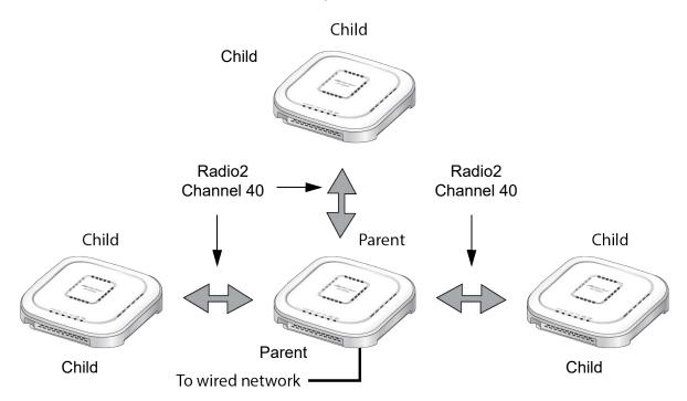
Figure 57. Example of Radio and Channel Assignments in a WDS Bridge
