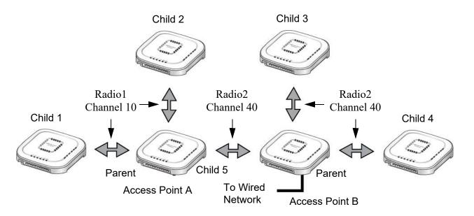
Figure 58. Example of an Access Point as Both Parent and Child
