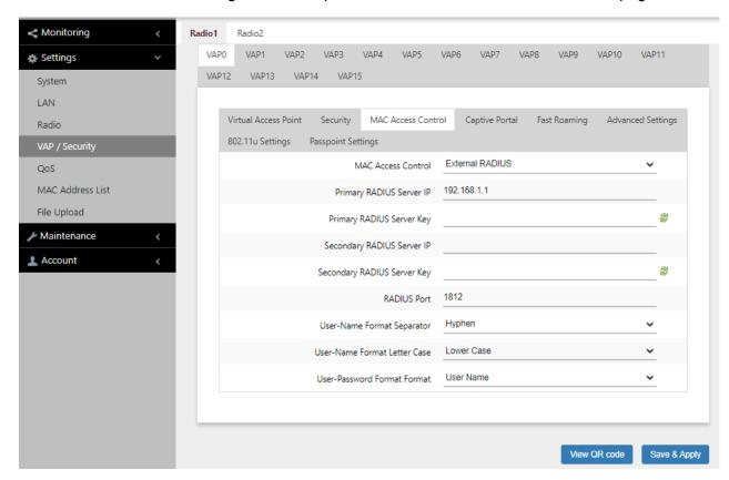
Figure 43. MAC Access Control - External RADIUS Window
