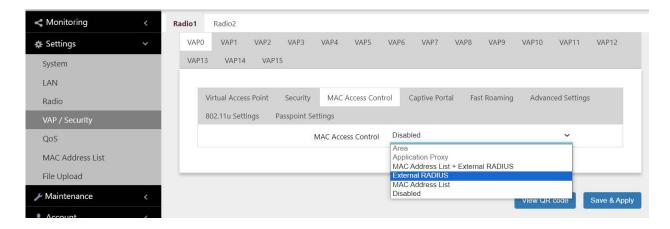
Figure 42. MAC Access Control - External RADIUS
