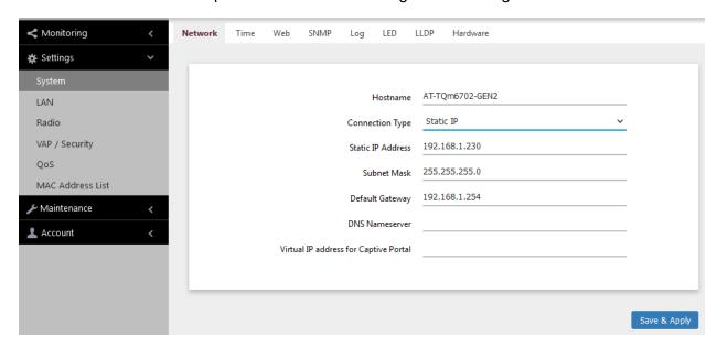
Figure 12. Network Window - Static IP Address
