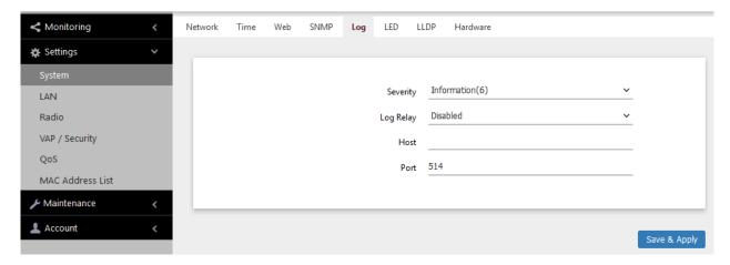
Figure 20. Log Window for Syslog Client
