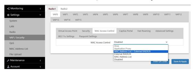
Figure 44. MAC Access Control - MAC Address List + External RADIUS
