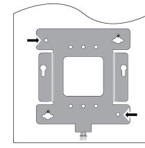
8. Install and tighten two M4 screws (not provided).
