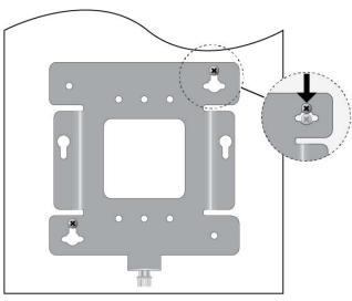
6. Tighten the screws snugly onto the bracket.
