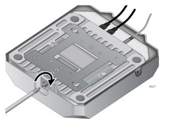
4. Place the Ethernet cable(s) and power cable (if any) along the cable guides inside of the top cover in the cable hiding space.
