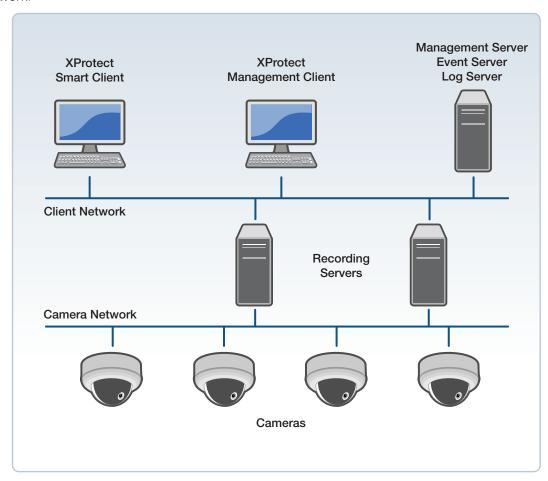
However, when using the Allied Telesis Plug-In to manage Allied Telesis PoE switches that are connected to the camera network, direct network connectivity is required between the switch and the machines that are hosting the XProtect Client software. To preserve network security and performance, it is recommended that separate VLANs be used on the switch for the management interface and the camera ports.
