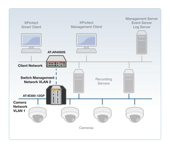
In the example above, the AR4050S UTM Firewall is used on the client network and the IE300-12GP PoE Switch is used on the camera network. If we suppose that port1.0.1 on the IE300 is connected directly to the AR4050S, and the client network is configured for the address range 192.168.15.0/24, the configuration for the IE300-12GP would be something like this:
