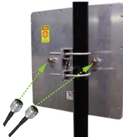
Figure 32. Installing Antennas to the Access Point
